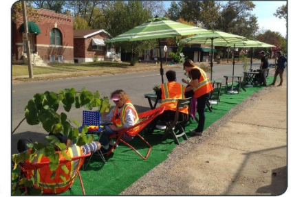
This "parklet" narrows the street in order to slow traffic and extends the sidewalk to provide more usable space for people to walk and spend time. Photo: Trailnet
